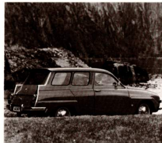
A slotted roof keeps dirt from collecting on the 95's rear window.
