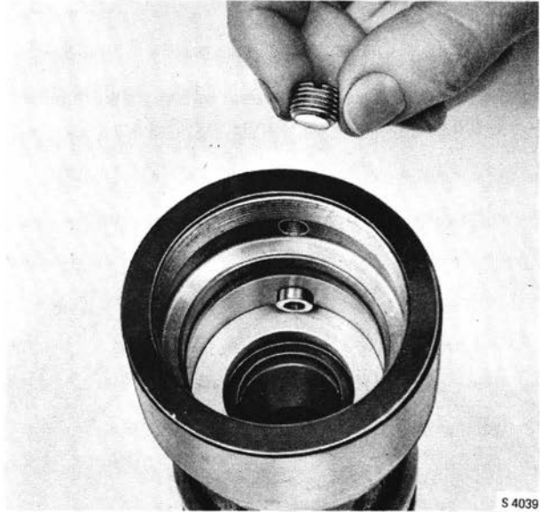
LOCKING THE CONE IN PLACE WITH A SPECIAL SCREW Tool 8995953
