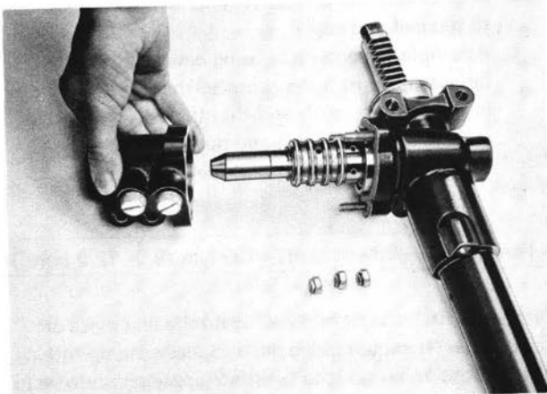
FITTING THE VALVE HOUSING. THE VALVE SHAFT IS FITTED WITH FITTING CONE 8995979
