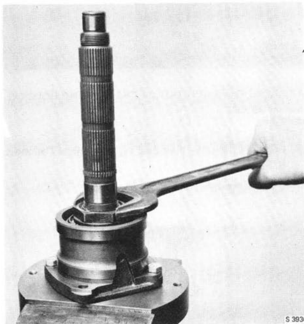
REMOVING THE PINION BEARING NUT Fixture 8790636, holder ring 8790651 and key 8790453
