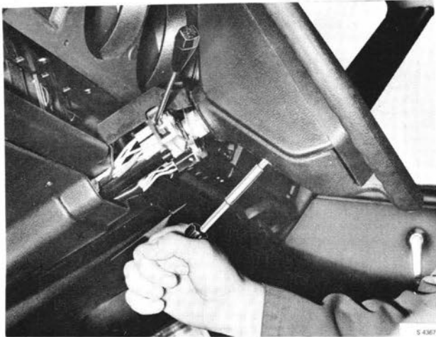
REMOVING THE SAFETY PAD
