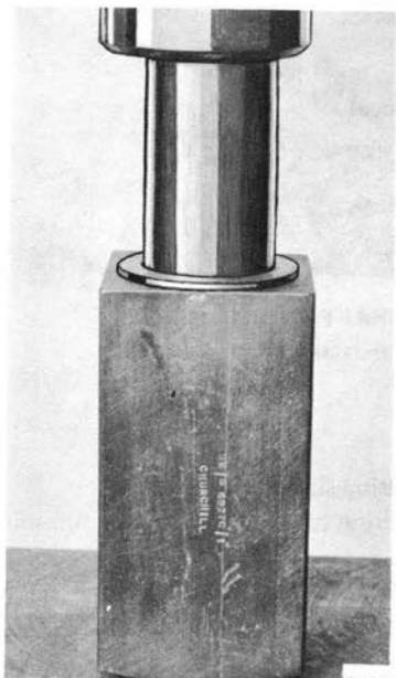
PRESSING THE PUMP SHAFT INTO THE BEARING HOUSING, UP TO AND INCL. MODEL 1976 Tools 8390544 and 8390551
