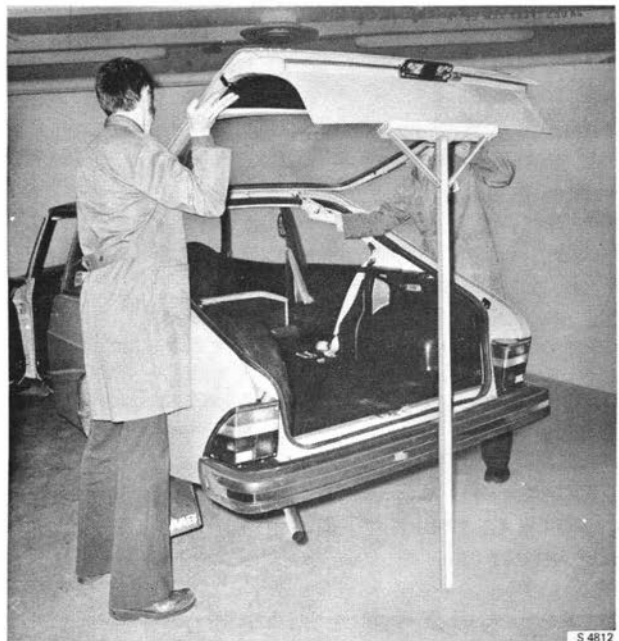
LIFTING OFF THE LUGGAGE COMPARTMENT DOOR
