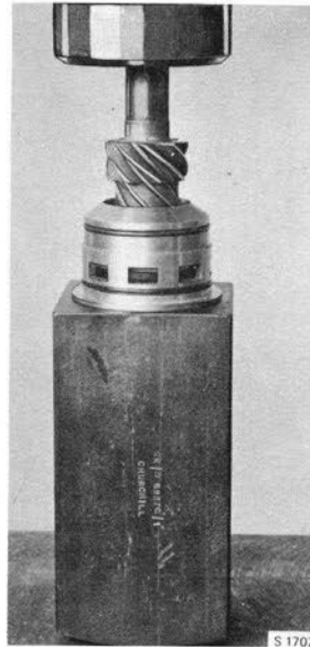
EXPPELLING THE PUMP SHAFT Tool 8390544
