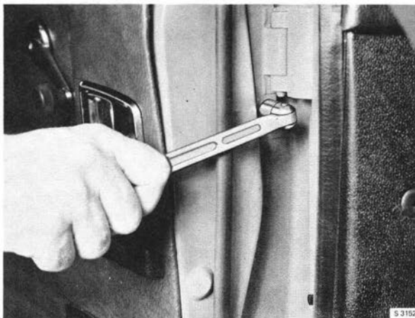
ADJUSTING VERTICAL AND FLUSH FIT OF REAR DOOR
