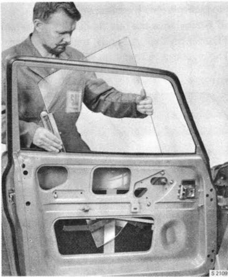
INSTALLING THE DOOR WINDOW
