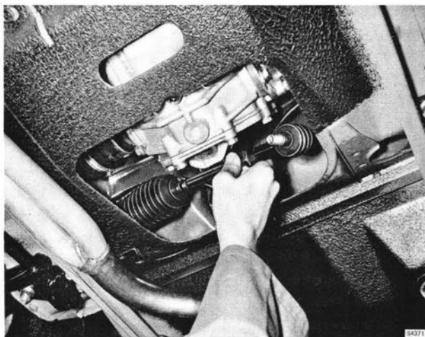
BENDING THE TIE ROD DOWN THROUGH THE OPENING IN THE BODY
