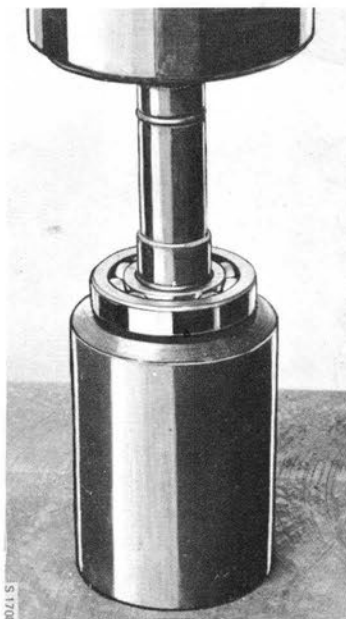
EXPPELLING THE SHAFT FROM THE BEARING Tool 8390536
