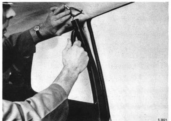
DOOR PILLAR PADS ARE MOVED INTO POSITION
