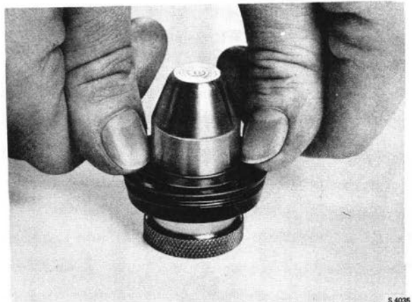
SLIDE THE SERVO SEAL ONTO THE FITTING SLEEVE USING THE FITTING CONE (SPECIAL TOOLS 8995938 AND 8995946)
