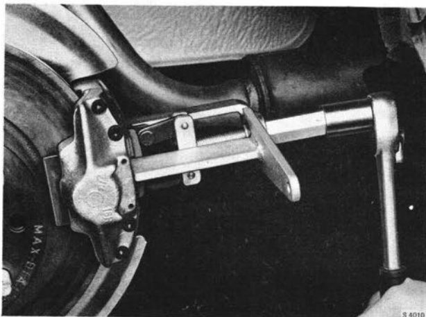
REMOVAL OF BRAKE PADS WITH EXTRACTOR 8995771
