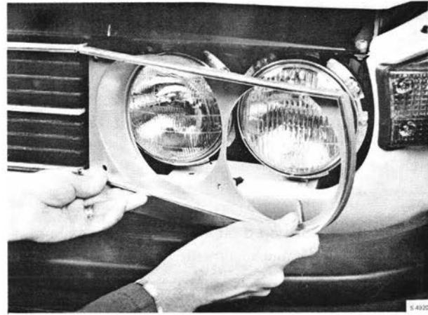
REMOVING THE HEADLIGHT TRIM FRAME
