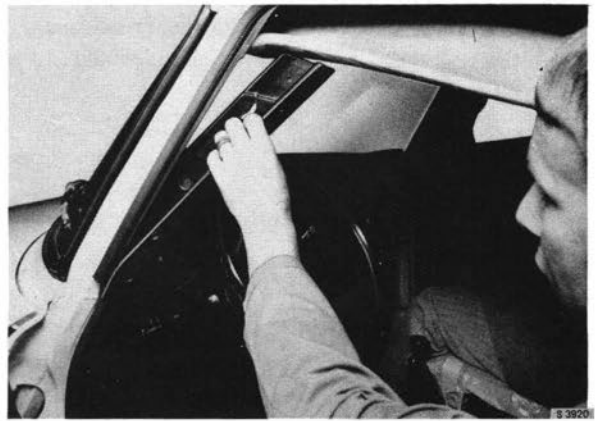
THE FRONT DOOR PILLAR PADS ARE INSTALLED
