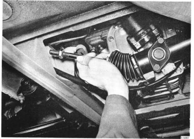
BEND THE LEFT TIE ROD DOWN THROUGH THE OPENING IN THE BODY
