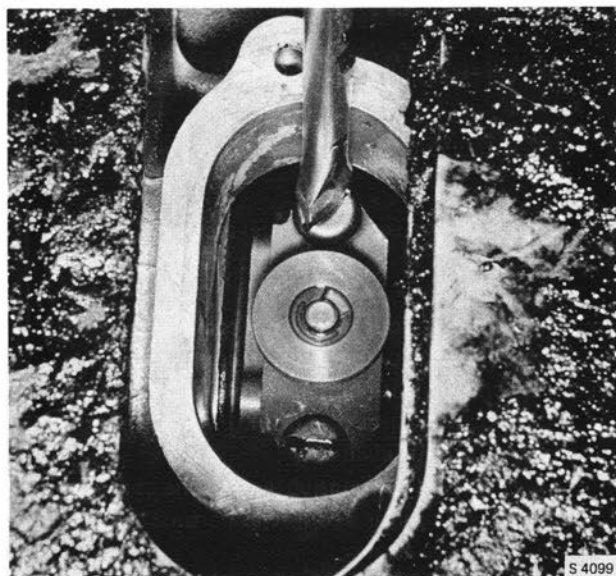
THE GOVERNOR SCREWS ARE REMOVED
