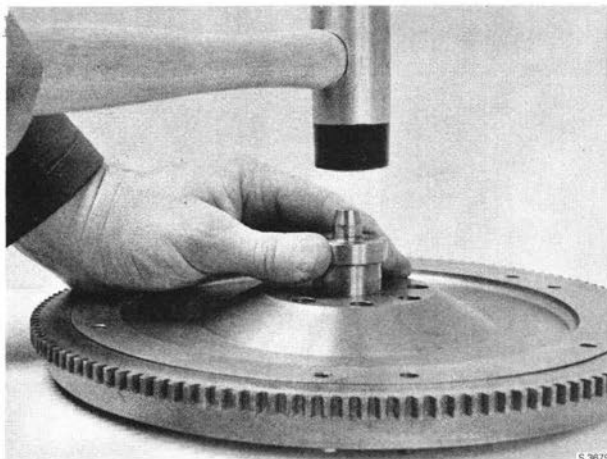
REMOVING THE CLUTCH SHAFT BEARING Tool 8391997
