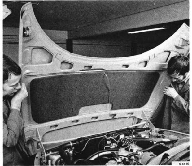
LIFTING OFF THE HOOD
