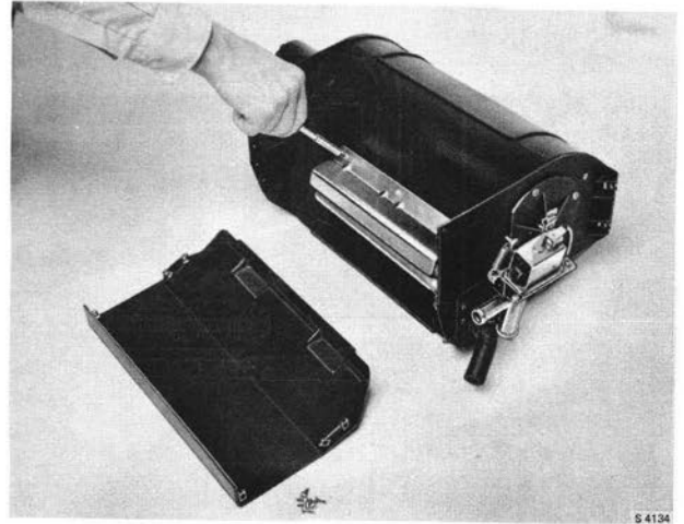
THE HEAT EXCHANGER RETAINING PLACE IS REMOVED
