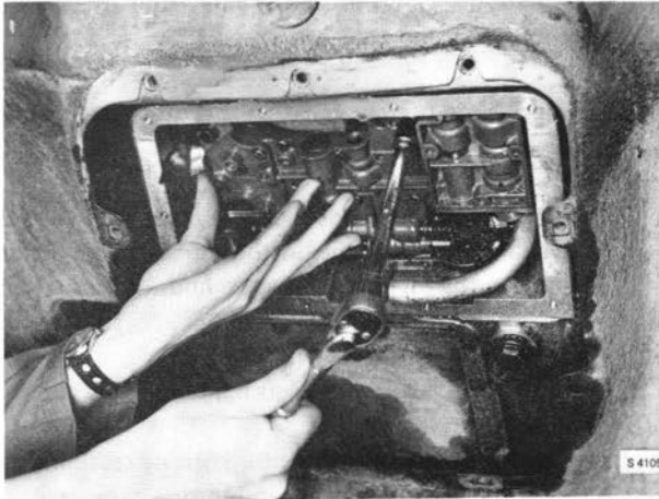
SCREWING ON THE VALVE HOUSING
