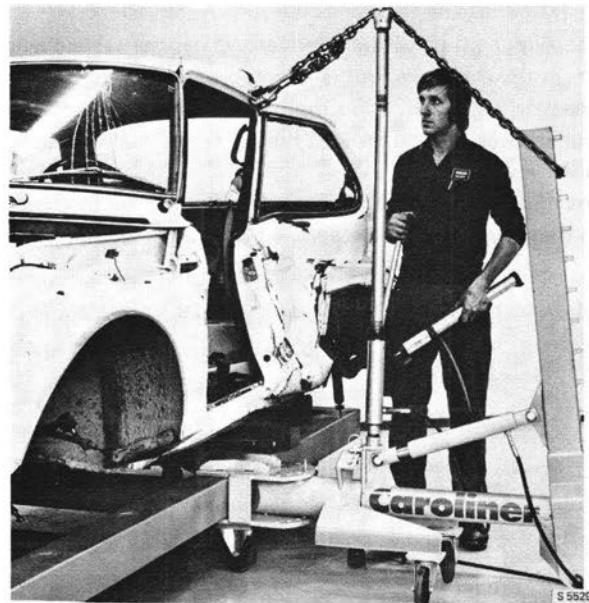
LOADS MAY BE APPLIED IN AN UPWARD DIRECTION BY MEANS OF AN ADDITIONAL HYDRAULIC CYLINDER AND AN EXTENSION PIECE
