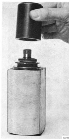
FITTING THE WATER PUMP SEAL, UP TO AND INCL. MODEL 1976 Tools 8390544 and 8390536
