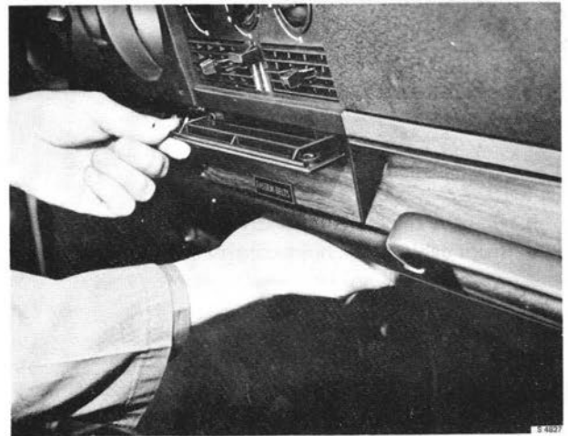
PUSHING OUT THE CENTER SECTION OF THE PANEL
