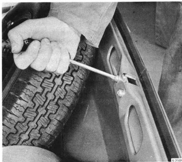
ADJUSTING THE STRIKER PLATE
