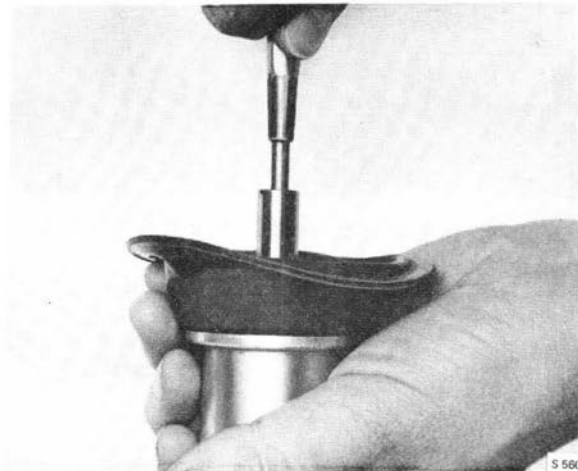
THE CIRCLIP IS PRESSED INTO THE PISTON
