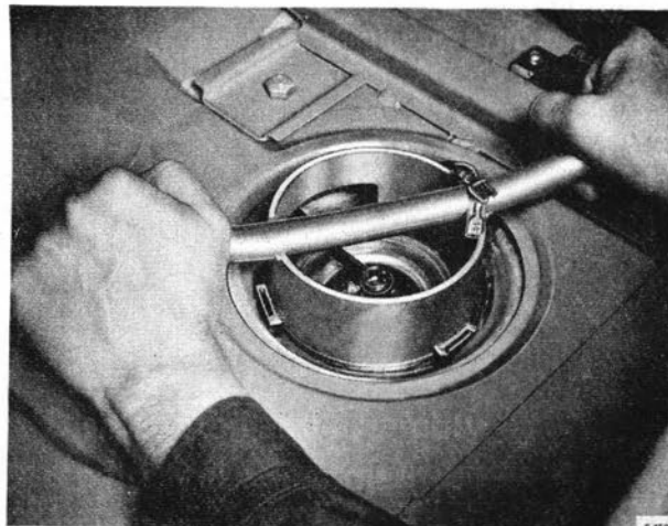
TURNING THE FUEL PUMP Tool 8392433
