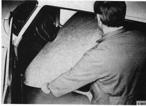
THE LINING IS LIFTED OUT THROUGH THE LEFT DOOR
