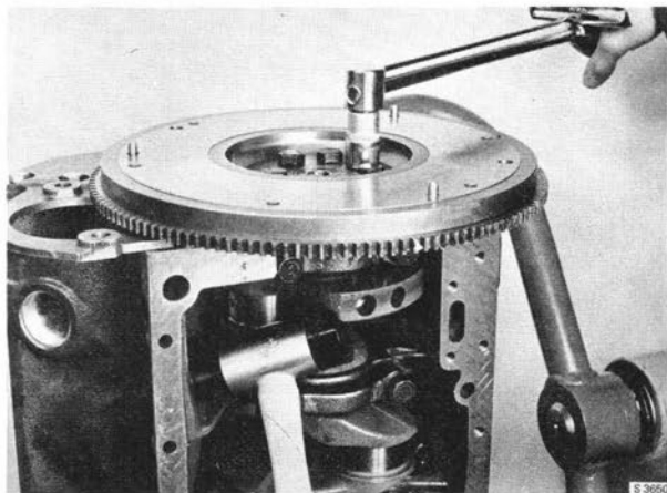
TIGHTEN THE FLYWHEEL SCREWS TO SPECIFIED TORQUE
