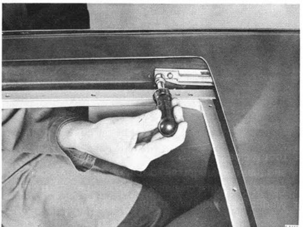
THE TWO SCREWS IN THE FRONT ENDS OF THE GUIDE RAILS ARE INSTALLED
