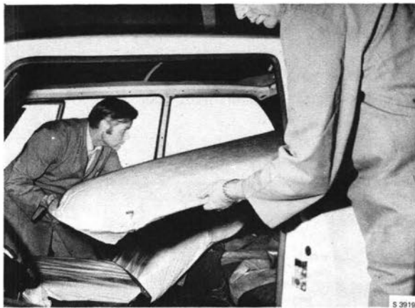
THE LINING IS MOVED IN POSITION
