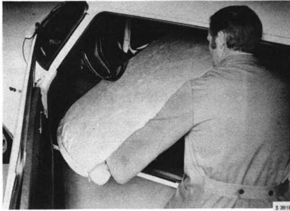
THE LINING IS LIFTED INTO THE CAR
