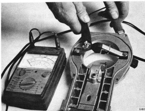
CHECKING THE STOP BRACKET INSULATION
