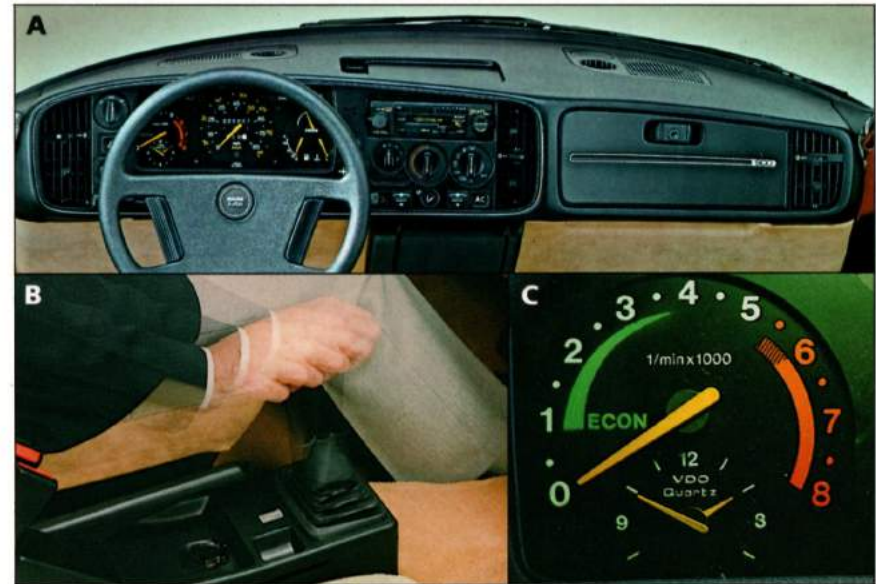
The 900's cockpit is designed to give the driver complete control. Figure A shows the dashboard with instruments displayed at the bottom edge of the driver's vision and controls close at hand. Figure B demonstrates "clustering" of controls by function; all of the starting controls (gearshift, ignition lock and handbrake) are located together at driver's right side. Figure C shows Saab's new tachometer with an indicator to show the most economical engine speeds.
