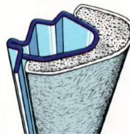
Roof pillars and windshield supports are covered with thick padding to absorb shock from bumps or collisions.
