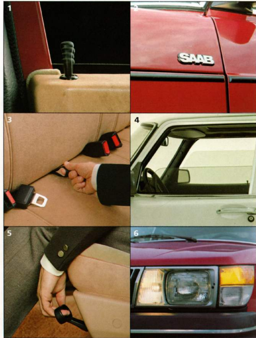
1: Central locking system for 900S/Turbo 3-door models. 2: Protective belt line molding. 3: Simplified latch and fold-down mechanism for rear seat. 4: Bronze-tinted windows. 5: Increased rearward travel for driver's seat. 6: New front parking lights.
