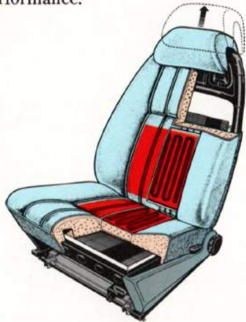
Firm padding, strong steel frames and polyester velour coverings combine to make one of the most comfortable and supportive car seats in the world. Saab seats are adjustable fore and aft; for seat height and angle; and for backrest rake. Front seats in the 900S and Turbo models are electrically heated.
