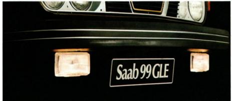
Fog lamps with halogen bulbs and yellow lenses are fitted under the front bumper.
