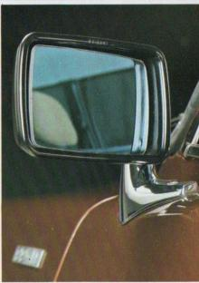
The outside rear-view mirrors can be controlled electrically by means of two switches on the control panel.
